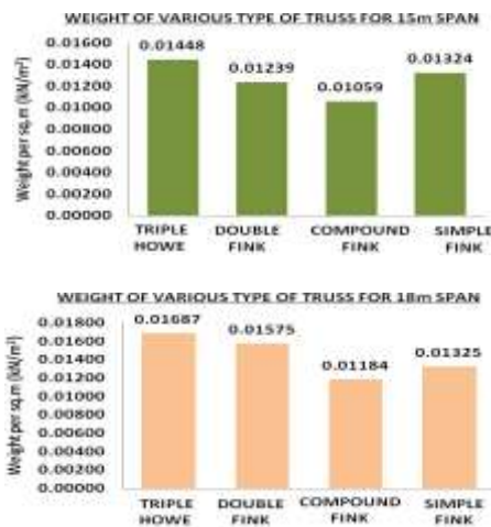
Chart 25: Graph showing weight of different types of truss for a given span.
