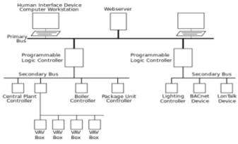
Fig -2: Building Automation System
