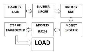
Fig.1: Block diagram representation of photovoltaic system.
