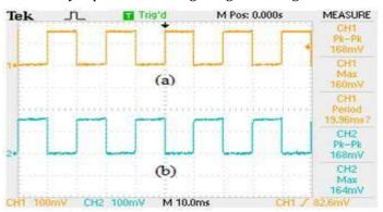
Fig 3: (a) Pin #10 output (b) pin #11 output of CD4047 Ic
