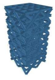
**Model V** – Steel diagrid with steel frame.
