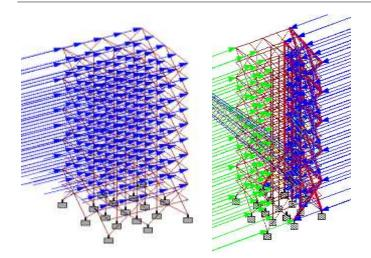
**Fig 2.3:** Application of earthquake and wind forces using STAAD- pro.
