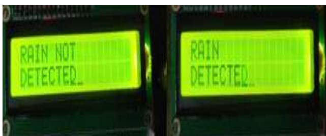
Fig 10-: Rain Detection results.
