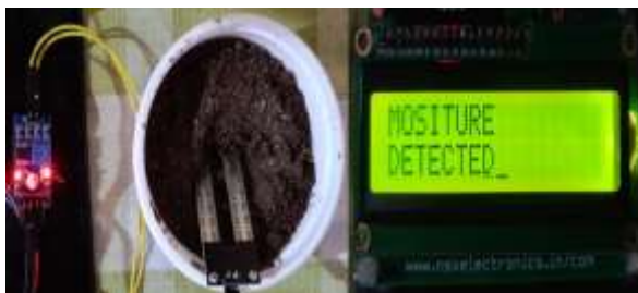
Fig 8-: Moisture detected when the sensor is in contact with any damp soil surface.
