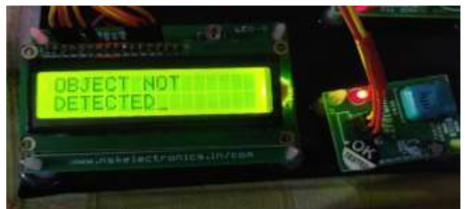
Fig -4: IR sensor without any Object Obstruction
