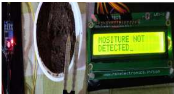
Fig -7: Moisture Undetected when the sensor is not in contact with any damp soil surface.
