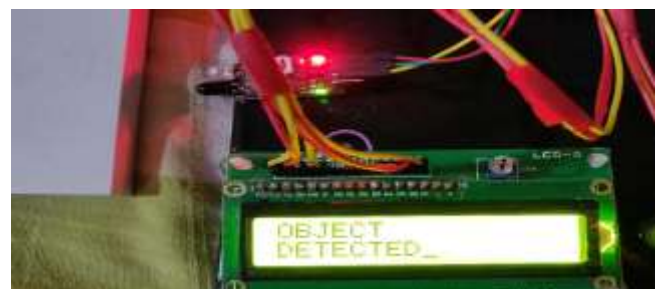
Fig -5: IR sensor output with Object Obstruction
