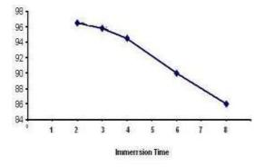
Fig.3 Variation of I.E in 1M H<sub>2</sub>SO<sub>4</sub>as mild steel at different immersion time of Pantoprazole.
