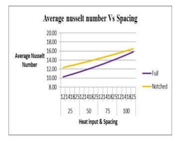
Fig.8 Graph of Average Nusselt numberVs Spacing
