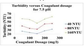
(d) Fig 1 (a,b,c,d): Residual turbidity v/s Coagulant dosage, Effect of coagulant dosage on clarification of water
