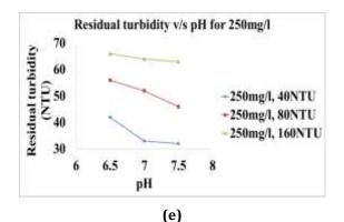
**Fig 2(a,b,c,d):** Residual turbidity v/s pH, Effect of pH on clarification of water
