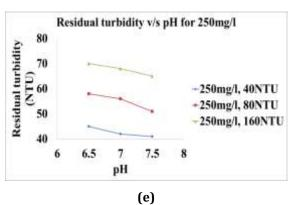
**Fig 5(a,b,c,d,e):** Residual turbidity v/s pH, Effect of pH on clarification of water
