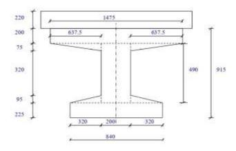
Fig 2: Girder at section 1
