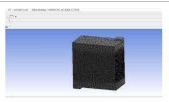
Fig (d):- Meshing of Chamber in which elliptical tubes are mounted.
