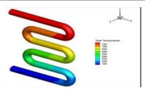
**Case (ii):** Thermal variation in receiver's tube having an elliptical cross-section.
