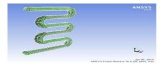
Fig (a): - Meshing of circular Section tube.
