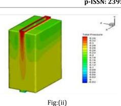
**Case (ii):** Elliptical section tube has installed inside the block.
