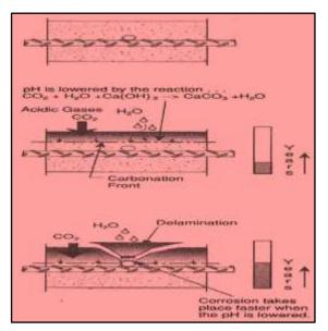
Fig.6 process of carbonation of concrete
