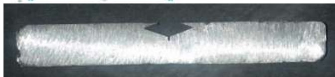
Figure 5: SENB specimen dimensions as per ASTM E399
