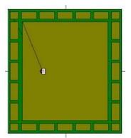
Fig 1(b) Geometry of Patch with EBG
