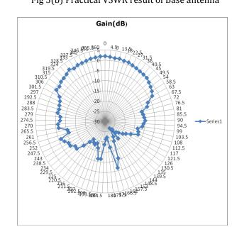
Fig 5(c) Practical Radiation pattern of Base antenna
