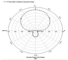
Fig 6(c) Gain plot in polar of patch With EBG
