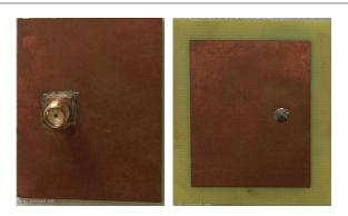
Fig 4(a) & 4 (b): Fabricated antennas with top view and bottom view of Basic microstrip antenna
