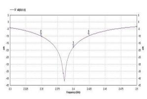
Fig 2(b) Simulated result of patch with EBG
