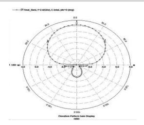
Fig 6(b) Gain plot in polar of Base antenna without EBG
