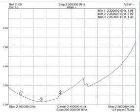
Fig 5(b) Practical VSWR result of Base antenna
