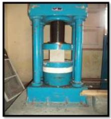
Fig 2 Comptressive strength test set up
