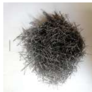
Fig-1 Crimped steel fiber
