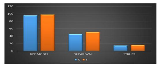
The displacement goes on increasing as the building height goes on increasing, this is also true when we provide Un-reinforced masonry(URM) shear walls in the building the displacement of the building decreases and further decrease by providing the struts in diagnol positions.
