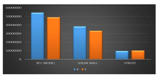
Story stiffness of the structures with URM shear wall is increased compared to bare frame (without shear wall)in X-direction. This increase in stiffness is due to increase in the seismic weight of the building
