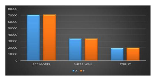
The drift when compared to that of the normal Rcc structure decreases when we provide shear walls and also when provided with struts. So at final by providing shear wall along with struts will be better model when compared with other
