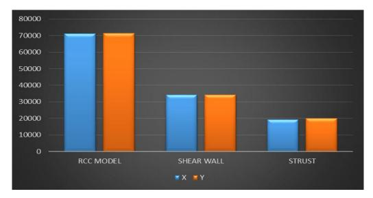
The stiffness when compared to that of the normal Rcc structure decreases when we provide shear walls and also when provided with struts. So at final by providing shear wall along with struts will be the better model when compared with other.
