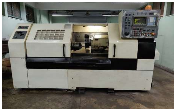
Fig.1 CNC ACE LT-20 Lathe machine used for performing Turning operation.
