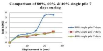
The load-settlement graph was drawn from the recorded data. The ultimate load for the 40%, 60% & 80% (5 cm) length of piles with 1D (2.5 cm) of 7 days curing was 4.90kN,8.16 &10.96 at 25 mm settlement.
