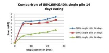
The load-settlement graph was drawn from the recorded data. The ultimate load for the SMP of 40% 60% &80% L/d ratio of 14 days curing was 4.06 7.16&8.10 KN at 25 mm settlement.
