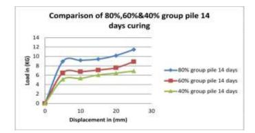
The load-settlement graph was drawn from the recorded data. The ultimate load for the 40%, 60% & 80% length of piles with 1D spacing of 14 days curing was 6.91kN, 8.90 &11.46 at 25mm settlement.
