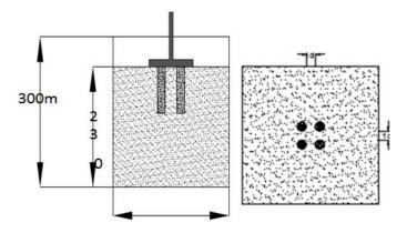
Fig 4.5 Typical diagram of 40% length of group piles resting on circular plate footing with 1D spacing.
