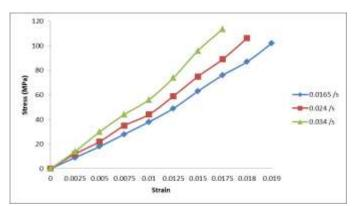
Chart-5 Stress-strain for 4.80mm thickness specimens
