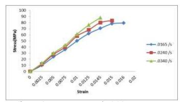
Chart-4 Stress-strain curves for 3.25 mm specimen
