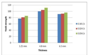
**Chart-12** Effect of thickness on yield strength of jute/glass hybrid composite material.
