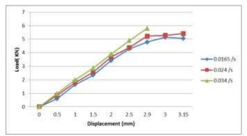
Chart-1 Load-Displacement for 3.25mm tensile specimens
