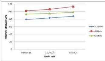
**Chart-13** Effect of strain rate on ultimate strength of jute/glass hybrid composite material.
