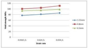
**Chart-11** Effect of strain rate on yield strength of jute/glass hybrid composite material
