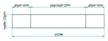
Fig 2. Standard tensile test specimen dimensions
