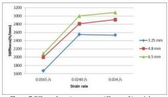
**Chart-7** Effect of strain rate on stiffness of jute/glass hybrid composite material.
