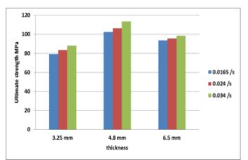
**Chart-14** Effect of thickness on ultimate strength of jute/glass hybrid composite material.
