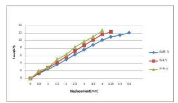
Chart-3 Load-Displacement for 6.5mm tensile specimens
