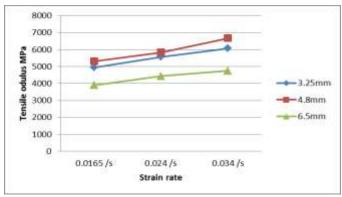
**Chart-9** Effect of strain rate on tensile modulus of jute/glass hybrid composite material
