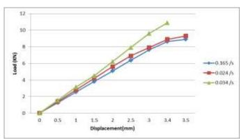
Chart-2 Load-Displacement for 4.8mm tensile specimen
