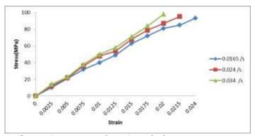
Chart-6 Stress-strain for 6.5mm thickness specimens
