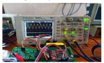
Figure 4.6: Triangular wave of 7 KHz
