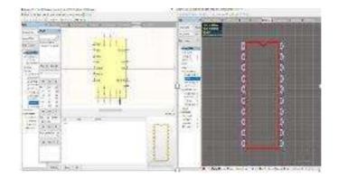
Figure 4.2: Footprint and symbol created for AD5620(DAC)
