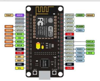
Fig. 4. Node MCU Pinout
