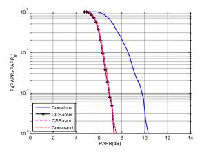
Fig.3.Comparison of the PAPR reduction performance between the conventional PTS scheme and the CSS scheme when N = 64
