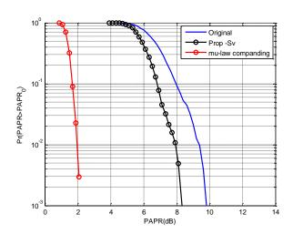
Fig. 5.Comparison of the PAPR reduction performance of the original OFDM, Proposed sv-sets and mu-law companding when N = 128, U = 4, and V = 4.
