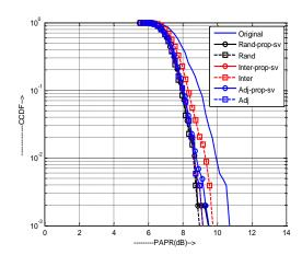
Fig. 4.Comparison of the PAPR reduction performance of the CSS scheme for three partition cases, which are random, interleaved, and adjacent partition cases when N = 128, U = 4, and V = 4 according to the used SV sets.
