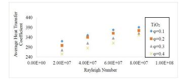
Fig 3 Variation of average heat transfer coefficient with particle concentration of  $TiO_2$
