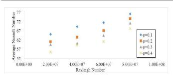
Fig 7 Variation of average nusselt number on particle concentration for AR=1/4
