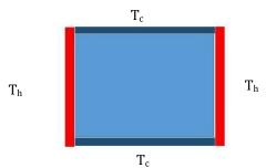
Fig 1 Flow configuration with horizontal walls are kept at  $T_{\rm c}$  and vertical walls are kept at  $T_{\rm h}$
