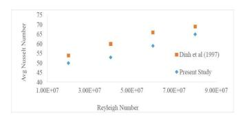
Fig 3. Variation of heat transfer coefficient with Rayeligh number
