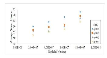
Fig 5 Variation of average Nusselt number with particle concentration of TiO<sub>2</sub>
