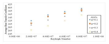
Fig. 4 Variation of average heat transfer coefficient with particle concentration of  $Al_2O_3$
