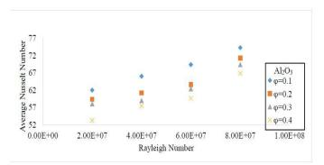
Fig 6 Variation of average Nusselt number with particle concentration of  $Al_2O_3$
