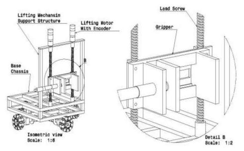
Figure 6: Detail Isometric View of Pneumatic Gripper
