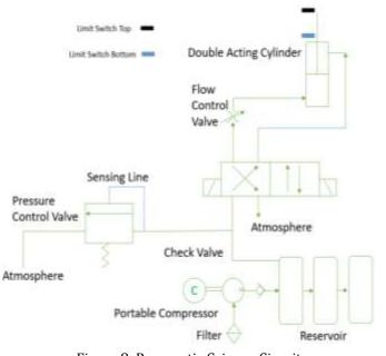
Figure 8: Pneumatic Gripper Circuit
