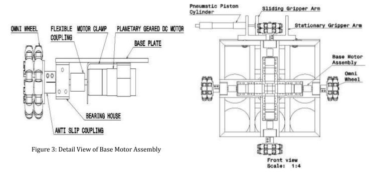
Figure 4: Base Motor Assembly
