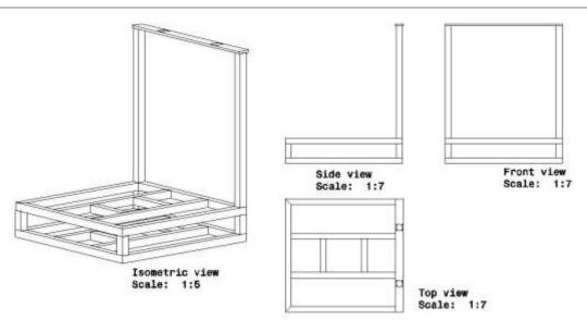
Figure 2: Isometric View of Chassis
