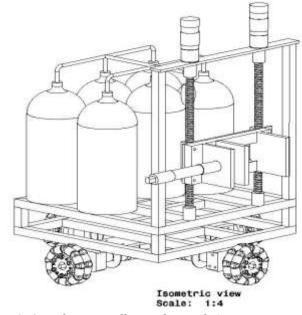
Figure 9: Complete Travelling Robot with Omni Directional Wheel
