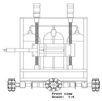
Figure 5: Vertical Motion Assembly
