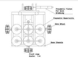
Figure 7: Pneumatic Gripper Assembly Top View
