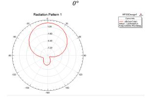
Fig 5(b):- Radiation Pattern of proposed antenna at  $\varphi = 0^{\circ}$
