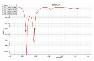
Fig 3(b):- Simulated result of reflection coefficient (S11) vs. frequency for proposed antenna.
