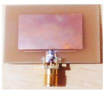
Fig 6:- Fabricated antenna
