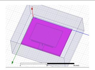
Fig 2(b):- Proposed Antenna design on the HFSS Software
