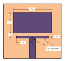
Fig1: - Geometry of the proposed wideband patch antenna.
