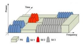
**Fig -1**: Concept of opportunistic spectrum sharing: secondary utilization of the identified spectrum holes.
