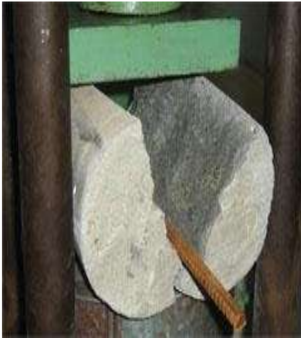
Figure 6: Split Tensile Strength Test
