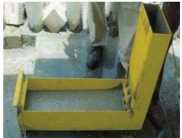
Figure 4: L Box Test
