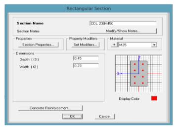
Figure 11: Column section details for all the columns in the structure
