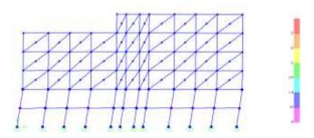
Figure 17: Load Resisting Mechanism for a typical frame of Building with Infill panels
