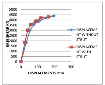
Graph 3: Base shear Vs Roof displacement curve for Building in Y direction IRJET
