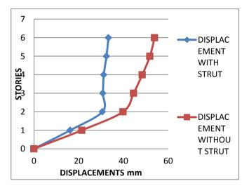
Graph 5: Displacement profile of Building at the formation of mechanism in Y direction
