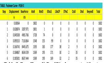
Table 3: Base Shear Vs Roof Displacement withoutInfill walls
