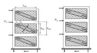
**Figure 1: Concentric Struts**
