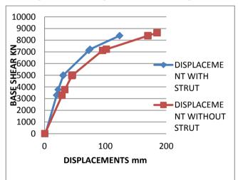
Graph 2: Base shear Vs Roof displacement curve for Building in X direction
