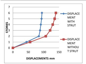
Graph 4: Displacement profile of Building at the formation of mechanism in X direction
