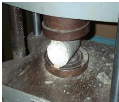
Fig 4.2: Split Tensile Strength Test
