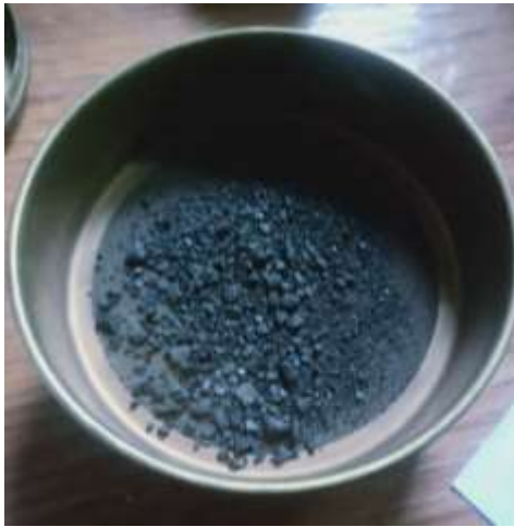
Fig-3: Obtained sieved coal sample after crushing by hammer
