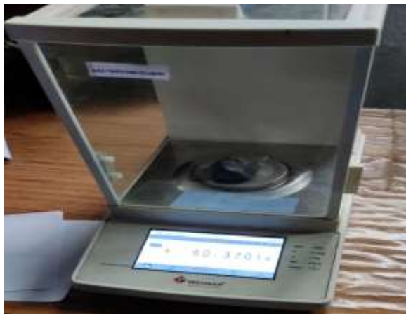
Fig-4: Weighting machine for measuring the weight of the coal sample
