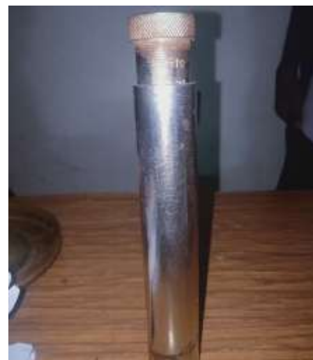
Fig-2: Volume meter device for measuring the height of the sample
