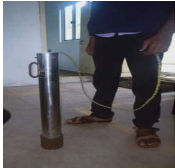
Fig-1: MS cylinder with rope wound hammer
