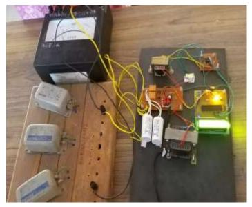
Fig -3: Hardware of Automatic Power Factor Control
