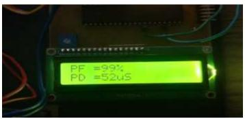
Fig 5. Showing corrected power factor on LCD
