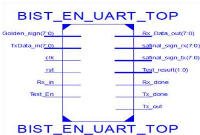
Figure 11 Top Module UART
