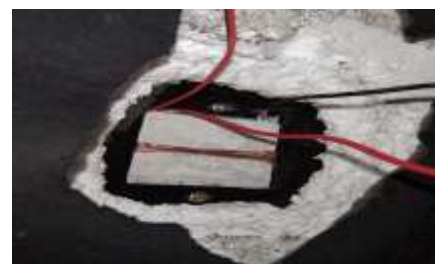
Fig 7. Peltier module inside the helmet
