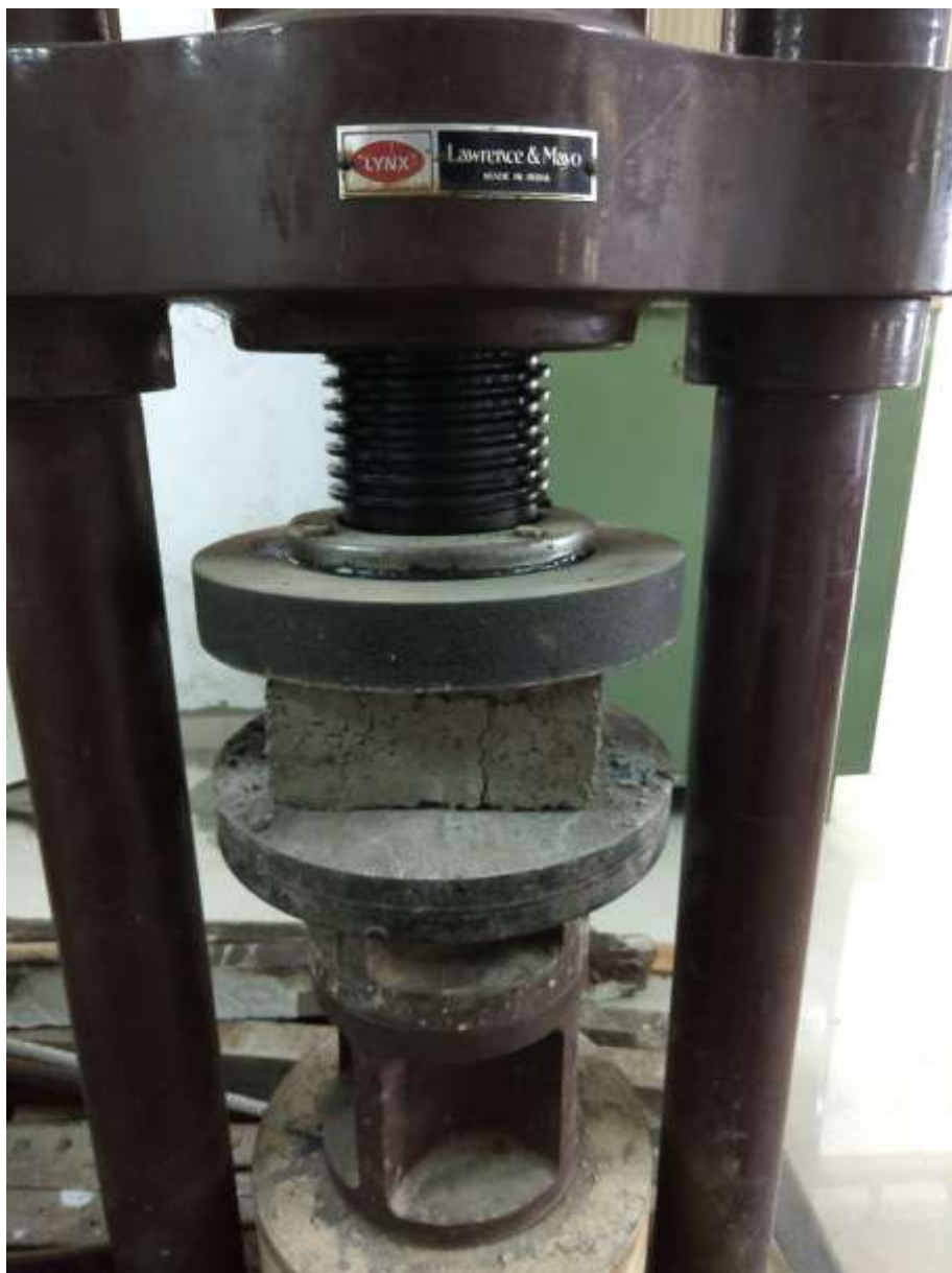
Fig. 2. compressive load testing on standard size mud brick of various ingredients
