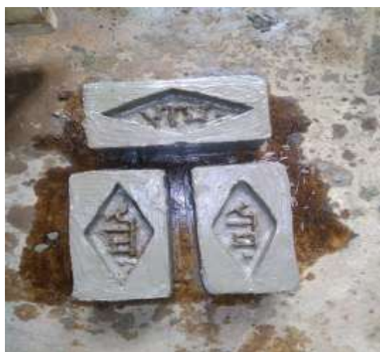
Fig 1. STANDARD SIZE MUD BRICK PREPARED FOR DRYING
