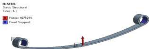
Fig. no.4 boundary condition of steel leaf spring
