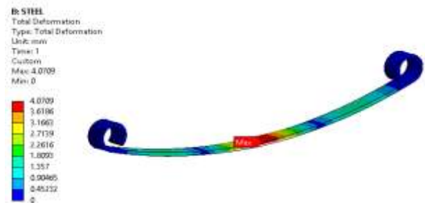
Fig. no.6 Total deformation of steel leaf spring
