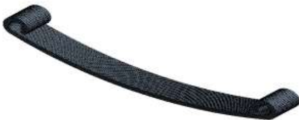
Fig. no.4 Meshing of steel leaf spring
