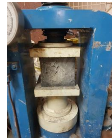
Fig1 Testing of cube in UTM machine
