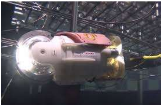
Fig.5: Mini Manbo (Sun Fish) Robot: Swimming Robot for Inspection
