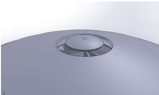
Fig- 5: Inlet section of OHV
