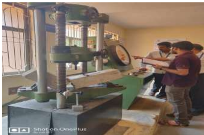
Figure 2: Photograph of Flexural Test(Broken beam)
