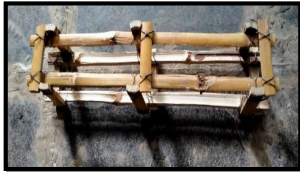
Fig: Bamboo Reinforcement
