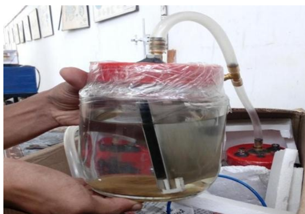
Fig -2: Oxy Hydrogen gas generative cell
