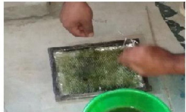
(b) During curing of the fiber plate
