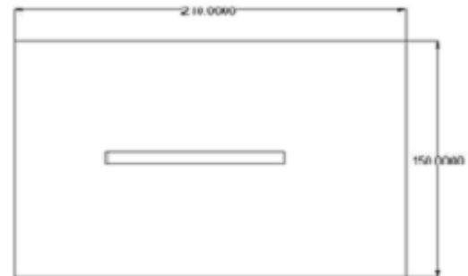
cover plate dimension 210x150x5
