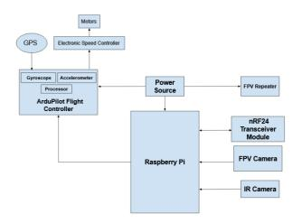
Fig -1. Block Diagram of the UAV system
