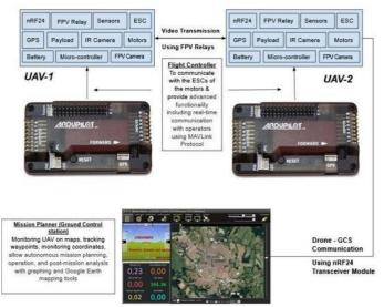
Fig -5: Overall interfacing of the flight controller with each other and the GCS
