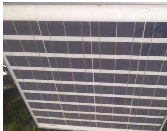
Figure.1 Dust laden PV panel
