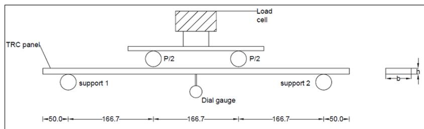
Fig -3: Schematic setup of four point bending test setup
