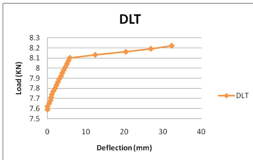
**Fig -5** Load vs. Deflection graph of DLT
