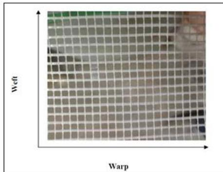
Fig -1: AR Glass fiber textile mesh
