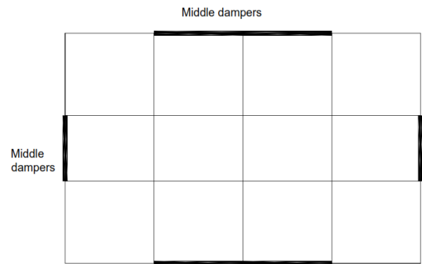
Fig -3: Building with middle damper system
