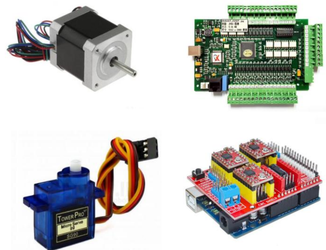
Fig -4: Hardware Components
