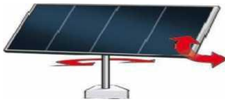
Fig.2. Dual axis tracker
