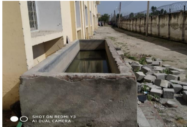
Figure 1 Curing of concrete for 7 days and 28 days
