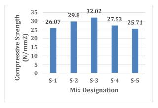
Graph-3: Cube Compressive Strength of Concrete with % of Copper Slag at 28 days curing period
